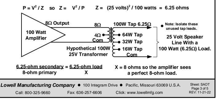
What if you want to use a transformer where the 25V tap power values don't perfectly match the power amplifier output rating?
