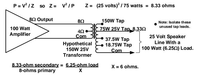
Because of the power rating of the amplifier, we know we don't want to load the transformer with more than 100 watts of 70V speakers (which we know will have a combined impedance of 6.25-ohms). The 8.33-ohm to 8-ohm winding ratio results in the amplifier seeing a 6-ohm load, which <u>will overload the 8-ohm output of the amplifier</u>.
