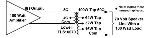
What if you want to use a transformer where the 70V tap power values don't perfectly match the power amplifier output rating?
