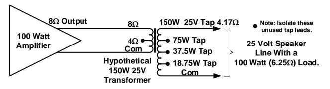
Because of the power rating of the amplifier, we know we don't want to load the transformer with more than 100 watts of 70V speakers (which we know from "Example 5" will have a combined impedance of 6.25-ohms). The 4.17-ohm to 8-ohm winding ratio results in the amplifier seeing an impedance as calculated below:
