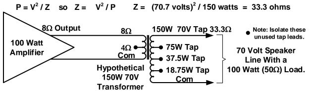
Because of the power rating of the amplifier, we know we don't want to load the transformer with more than 100 watts of 70V speakers (which we know from "Example 1" will have a combined impedance of 50 ohms). The 33.3-ohm to 8-ohm winding ratio results in the amplifier seeing an impedance as calculated below:
