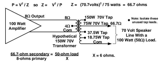
Because of the power rating of the amplifier, we know we don't want to load the transformer with more than 100 watts of 70V speakers (which we know will have a combined impedance of 50 ohms). The 66.7-ohm to 8-ohm winding ratio results in the amplifier seeing a 6-ohm load, which <u>will overload the 8-ohm output of the amplifier</u>.
