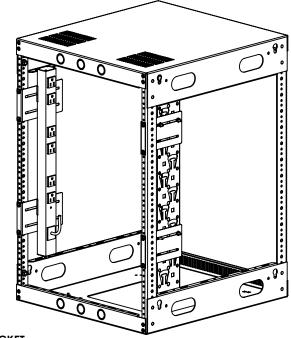
0 0 1/2" SCREW O Ø 0 **2U BRACKET** VERTICAL CABLE MANAGER: ATTACH (2) MOUNTING BRACKETS TO RAIL WITH (4) 10-32 X 3/4" RACK SCREWS. MANAGER MOUNTING THE MANAGER TO THE BRACKETS: ATTACH WITH (4) 10-32 X 1/2" SCREWS & KEPS NUT (2 ON EACH BRACKET) ۰Ĥ (Si) 0 P/N 24083 1-14-21 SHEET 1 OF 2
