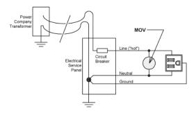
When everything is working normally and the AC line voltage is at the proper level, then the MOV isn't doing anything, it's as if it were an open switch.
