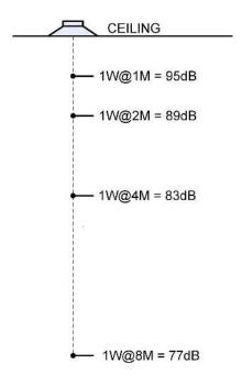
So what if we adjust the input power to more than 1W? The formula for SPL as is relates to input power is:
