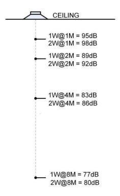
These formulas can be combined so that both input power and distance calculations can be done at the same time. This formula handles any power input at any distance.
