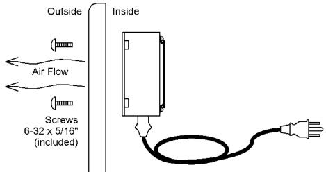
NOTE 1: If reverse airflow is required, remove fan mounting screws, flip fans over, and reassemble.
