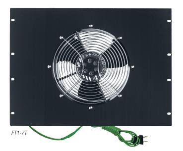
Ready-to-install 16-gauge steel panel with 10" dia. x 3.75"D tubeaxial fan with front and rear fan guards. This powerful turbo fan has feathered edges for lower noise. Includes green "thermo-cord" which has an integral thermostat probe to control fan activation and ensure efficient operation while saving wear and tear on the unit.
