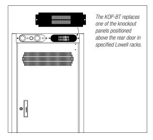
Steel panel with dual blower fans is made to replace a rear knockout panel in select Lowell racks. Air is pulled in from top/bottom fans, then blown out through vents. Includes power supply and thermostat probe controls fan operation automatically.
