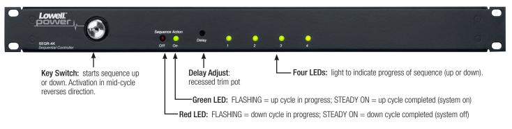
The low voltage rackmount sequencer is used in conjunction with remote power controls (RPCs) to provide time-delayed activation and deactivation of connected equipment, often located in another rack, room or building. The sequencer can also control accessory systems such as projector screens, lighting or blinds. To initiate sequencing, use the rocker switch on the front panel or connect an external switch to the rear terminal block for remote activation.
