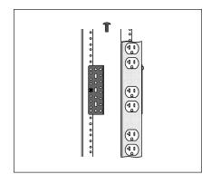
RACK w/ ADJUSTABLE RAILS (rear mount): Mount to rear rail with universal brackets, 10-32 screws.
