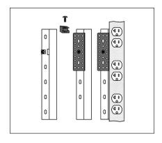
RACK w/ FIXED POSITION RAILS (and rear Z-angle bracket): Mount to Z-angle with universal brackets, 10-32 screws, cage nuts.
