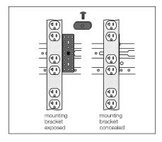
RACK w/ ADJUSTABLE RAILS (side mount): Mount to horizontal side supports with universal brackets, 1/4"-20 screws, flat nuts.
