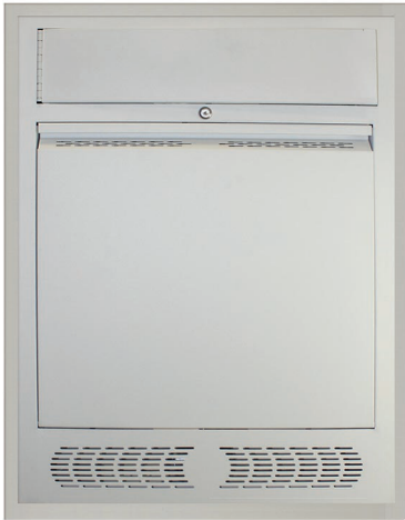
Wall-mount rack with two bays—a hinged pocket door on the upper bay swings open, the lower bay tilts down when opening to the service position (oil-filled dampers control the rate of descent).
