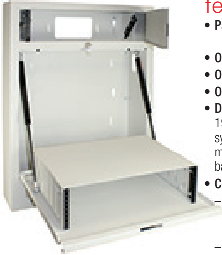
Wall-mount rack with two bays—a hinged pocket door on the upper bay swings open, the lower bay tilts down when opening to the service position (oil-filled dampers control the rate of descent).
