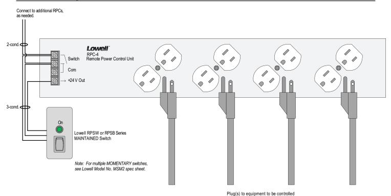
Wiring notes: Connections are made via 3-conductor cable (mic line works nicely, use shield as common).
