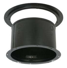
INSTALLATION: Recessed FOR SPEAKER SIZE: 8" EIA FOR GRILLE TYPE: Screw-mount or Torsion For use with an 8" speaker and torsion or screw-mount grille, the blind-mount enclosure includes a steel backbox and a plastic mounting ring. It's ideally suited for drywall or plaster ceilings that require a recessed enclosure to be installed from below because above-ceiling access is not available.
