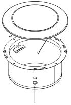
Knockouts: 1/2"–3/4" (combination) for conduit 1/2" for wire access
