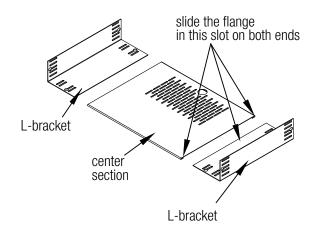
2. Position the shelf assembly just behind the front flange of the mounting rails and extend the L-brackets out to the inside of the other flange on the mounting rails. Align the slots in the L-brackets with the holes in the mounting rails and insert a 10-32 screw and nut in each hole.
