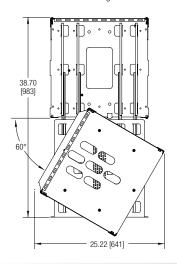
Rack slides forward on four support rails in base, then
