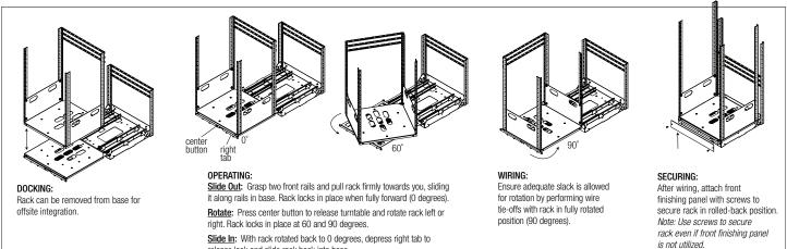
release lock and slide rack back into base.
