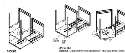
Rack can be removed from base for offsite integration.
