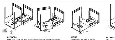
Slide Out: Grasp two front rails and pull rack firmly towards you, sliding it along rails in base. Rack locks in place when fully forward (0 degrees). Rotate: Press center button to release turntable and rotate rack left or
