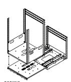
DOCKING: Rack can be removed from base for offsite integration.
