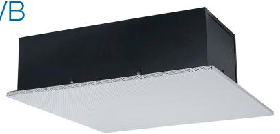
LT SERIES SPEAKERS are pro systems made for quick installation in suspended lay-in tile ceilings. The 2x2 assembly replaces a 2x2 ceiling tile. This model features a premium 8-inch coaxial driver, 70V 32W transformer, 2x2 grille with subplate and 0.8-cu.ft. volume backbox.
