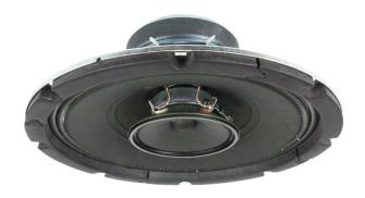
THE CT830A HIGH-PERFORMANCE DRIVER features a post-mounted, coaxially positioned tweeter for improved performance over traditional full-range (dual cone) speaker. The 3-inch tweeter provides wide dispersion in the high frequency range, enhancing speech/music intelligibility areas between speakers. This model is an outstanding choice for quality paging, public address, and background music applications that demand accurate voice/music reproduction.
