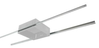
Channel rails distribute the weight of a speaker assembly to the ceiling support structure, reducing the likelihood of (2' x 2' or 2' x 4') tiles sagging under the weight of the speaker, which helps maintain the overall aesthetics of the installation. Channel rails are often required by local building codes for safety purposes.
