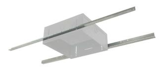
Channel rails distribute the weight of a speaker assembly to the ceiling support structure, reducing the likelihood of (2' x 2' or 2' x 4') tiles sagging under the weight of the speaker, which helps maintain the overall aesthetics of the installation. Channel rails are often required by local building codes for safety purposes.
