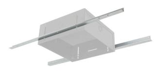
Channel rails distribute the weight of a speaker assembly to the ceiling support structure, reducing the likelihood of (2' x 2' or 2' x 4') tiles sagging under the weight of the speaker, which helps maintain the overall aesthetics of the installation. Channel rails are often required by local building codes for safety purposes.
