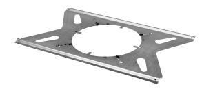
A tile-bridge distributes the weight of a speaker assembly to the ceiling support structure in a suspended 2' x 2' or 2' x 4' tile ceiling, reducing the likelihood of tiles sagging under the weight of the speaker, and helping to maintain the overall aesthetics of the installation. Tile-bridges are often required by local building codes for safety purposes. The LBS8-R1 can be used with or without a backbox depending on local building codes and the style and weight of the speaker assembly.
