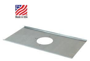
A tile-bridge distributes the weight of a speaker assembly to the ceiling support structure in a suspended 2' x 2' or 2' x 4' tile ceiling, reducing the likelihood of tiles sagging under the weight of the speaker, and helping to maintain the overall aesthetics of the installation. Tile-bridges are often required by local building codes for safety purposes. Model LBS4-DX tile-bridge requires an enclosure (backbox) and can be used with a screw-mount or torsion grille (with appropriate enclosure).
