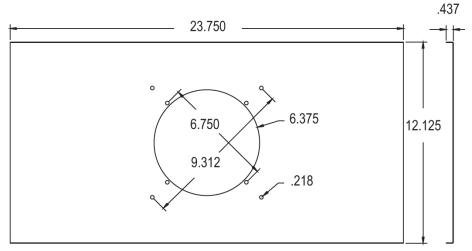
The outer holes are for use with backbox model DX104 or DX104-T. The inner holes are for use with backbox model CP4.
