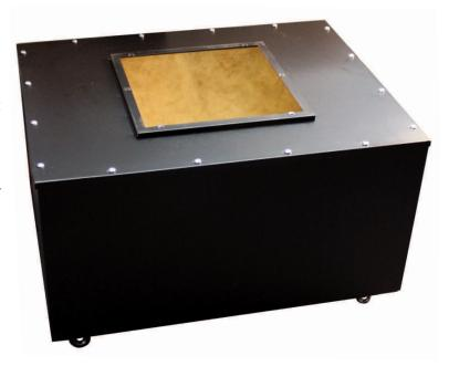
Backbox shall measure 23.25" x 30" x 15" with an internal volume of 5.9 cu.ft. It shall have four 1/2"–3/4" knockouts for conduit and 1/4"–20 forged eyebolts for suspended installation (using flyware by others). It shall be finished in black powder epoxy.
