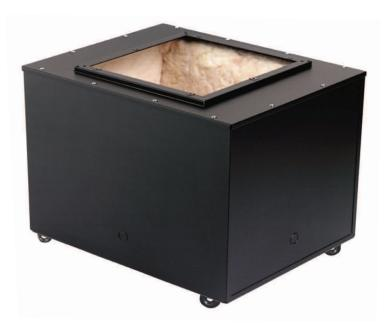
Backbox shall measure 23.25" x 18.25" x 16.75" with an internal volume of 4.0 cu.ft. It shall have four 1/2"-3/4" knockouts for conduit and 1/4"-20 forged eyebolts for suspended installation (using flyware by others). It shall be finished in black powder epoxy.
