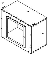
Welded tabs for channel rail support
