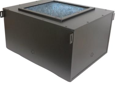
thick acoustic fiberboard and 1.5" thick acoustic lining. Backbox shall measure 23.25" x 18.25" x 12" with an internal volume of 2.9 cu.ft. It shall have four 1/2"–3/4" knockouts for conduit and two sets of slotted tabs welded on parallel sides for channel mounting or seismic anchoring. It shall be finished in black powder epoxy.
