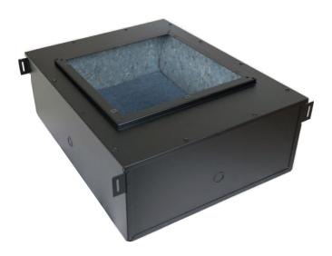
thick acoustic fiberboard and 1.5" thick acoustic lining. Backbox shall measure 23.25" x 18.25" x 8" with internal volume of 1.9 cu.ft. It shall have four 1/2"-3/4" knockouts for conduit and two sets of slotted tabs welded on parallel sides for channel mounting or seismic anchoring. It shall be finished in black powder epoxy.
