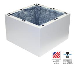
INSTALLATION: Surface-mount FOR SPEAKER SIZE: 8" EIA FOR GRILLE TYPE: Screw-mount Large volume surface-mount steel enclosure for ceiling or wall installation is designed to mount a screw-mount grille with a standard 8" speaker. The clean square format is ideal for schools, offices, restaurants, hotels and similar venues. Thick acoustic lining allows the speaker to operate at a more optimum loading level and provide the system with improved low frequency response.
