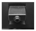
TERMINAL COVER: Incoming wire enters through the weather-resistant terminal cover and is protected by a rubber grommet. Maximum recommended wire size is 14AWG stranded. *Note: The grommet can be removed if larger wire sizes are used.*
